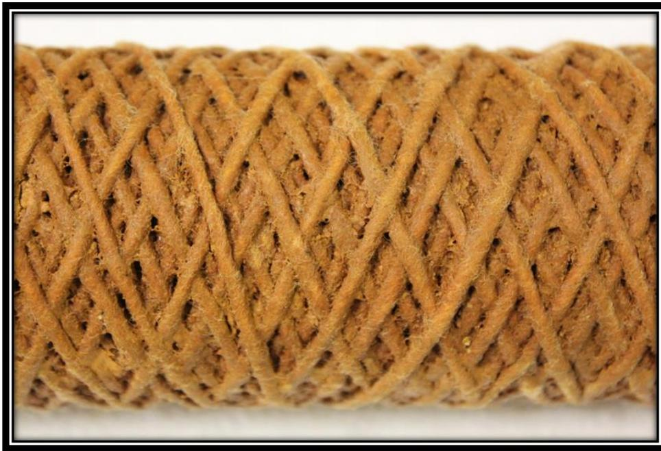
**Figure 7: Cartridge filter from pretreatment is heavily fouled with iron.**
