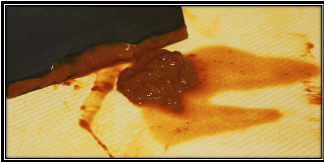
**Figure 3: Foulant collected from tail element membrane surface during autopsy.**
