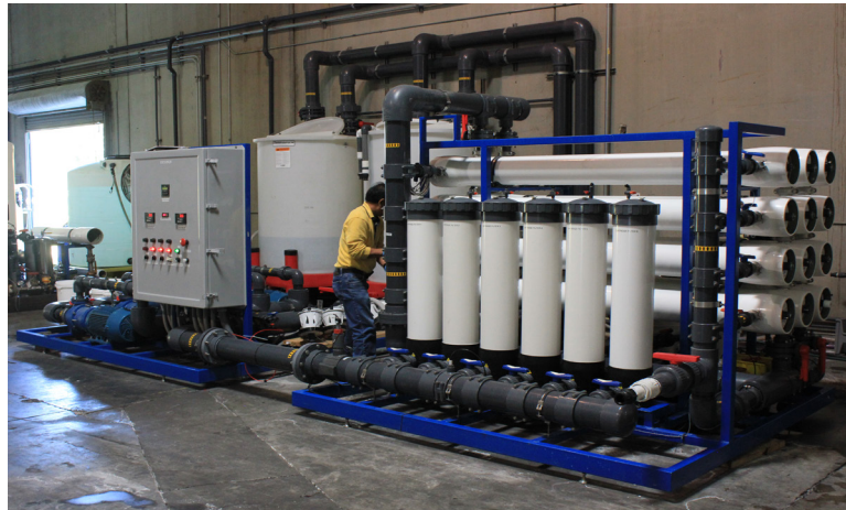
Two cleaning stations allow for simultaneous cleaning of up to 30 elements
