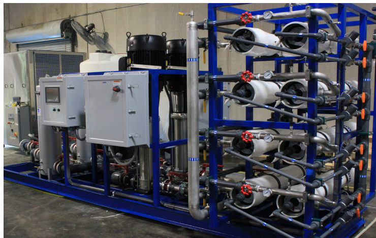
Test station designed for simultaneous testing of up to 8 elements
